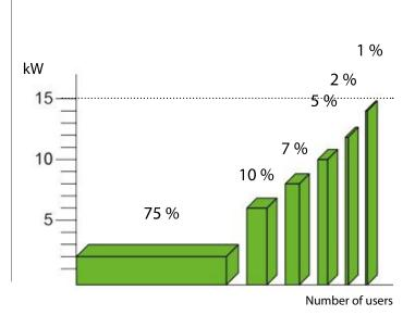
With a 15 kW vacuum producer with DC Green System the rpm and energy use is matched with the number of people using the system at the same time.
